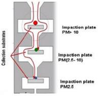
Fig. 1: Impactor working principle
