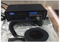
Fig. 4: EEL43M Smoke Stain Reflectometer (SSR)
